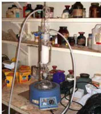
Fig. 9: Soxhlet Continuous extraction unit
