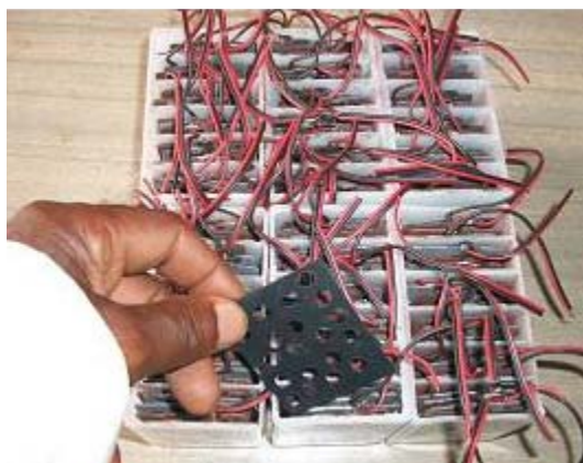
Fig. 12: Insulator being placed in a cell component, with the tapping electrodes already positioned.
