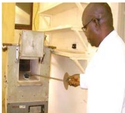
Fig. 11: Removal of organic constituents to obtain active inorganic sulphite.
